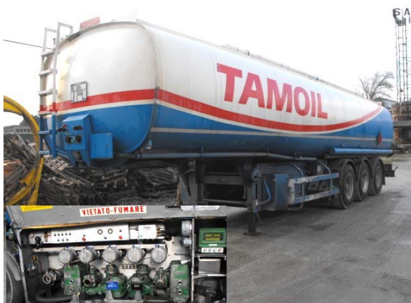
39.000 liters, 5 compartments, 4" bottom loading 27-AB3793
