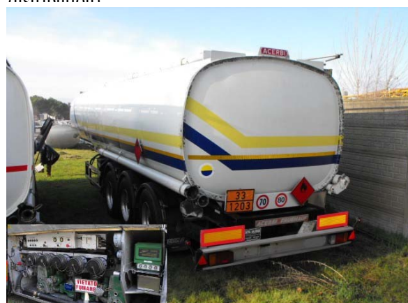
39.000 liters, 5 compartments, 4" bottom loading 27-AB3758
