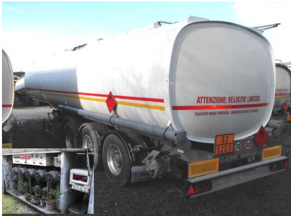
39.000 liters, 5 compartments, 4" bottom loading 27-AB907
