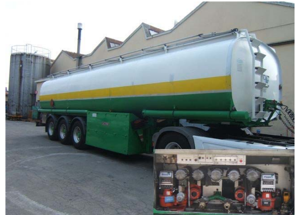
39.000 liters, 5 compartments, 4" bottom loading 27-AB304
