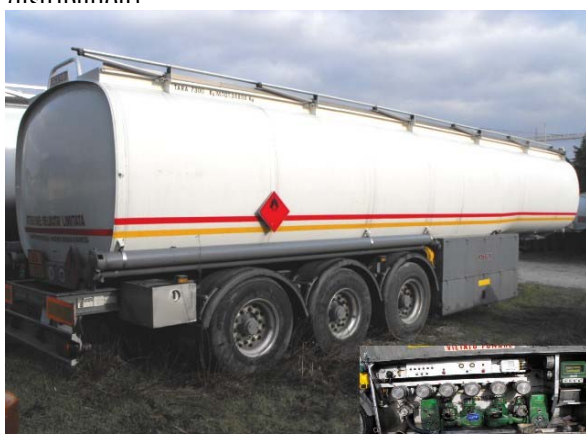
39.000 liters, 5 compartments, 4" bottom loading 27-AB3756
