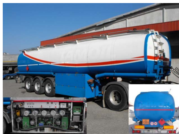
39.000 liters, 5 compartments, 4" bottom loading 27-AA9080
