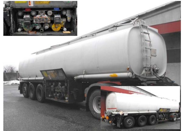
37.000 liters, 4 compartments, 4" bottom loading 27-GE245
