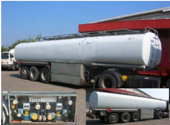
37.000 liters, 4 compartments, 4" bottom loading 27-SR541
