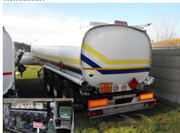
39.000 liters, 5 compartments, 4" bottom loading 27-AB3759
