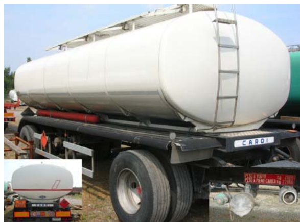
2 axles trailer, pneumatic suspension 22-TS103 19.580 liters aluminium tank, 4" bottom loading
