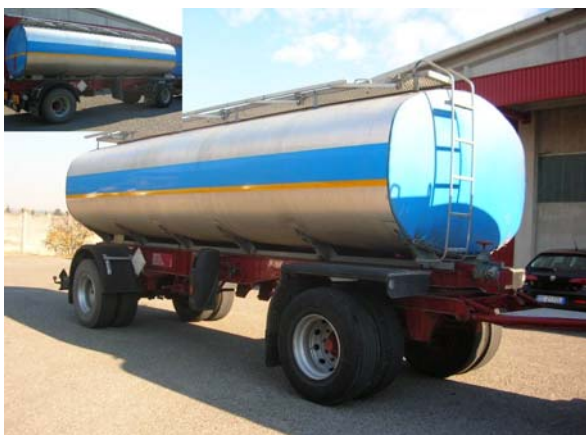
2 axles trailer, mechanic suspension 22-FO190 19.640 liters steel tank with cover fot hot product
