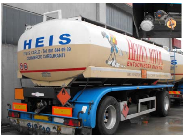
2 axles trailer, pneumatic suspension, ABS 22-AA910 18.250 liters aluminium tank, 4" bottom loading, ADR
