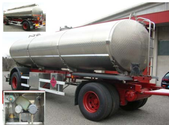
2 axles trailer, mechanic suspension 22-AL219 20.800 liters inox tank, 4" bottom loading, ABS, ADR
