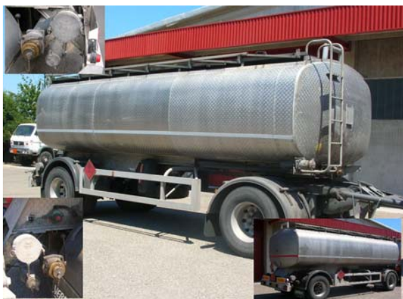
2 axles trailer, pneumatic suspension 22-AA657 21.950 liters aluminium tank ,4" bottom loading, ABS, ADR
