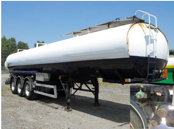
39.020 liters 1 compartment. 26-AL210 Pneumatic suspension, 6 tyres, ABS, ADR (primary transport)
