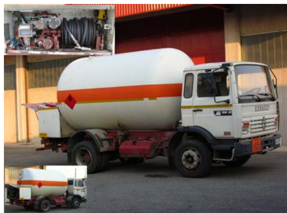
RENAULT M-160 14-GED767 10.800 liters, pump, mechanic litters counters, reel hose
