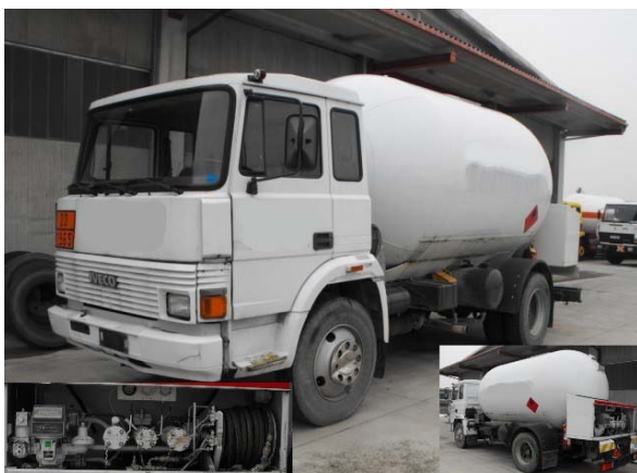
IVECO 135.17 14-BSD103 13.500 liters, pump, mechanic litters counters, reel hose
