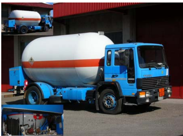
VOLVO FL616 14-AT329 15.800 liters, pump, mechanic litters counters, reel hose
