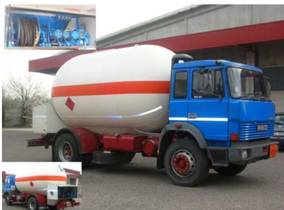
IVECO 175.24 14-BGB037 17.100 liters, pump, mechanic liters counters, reel hose
