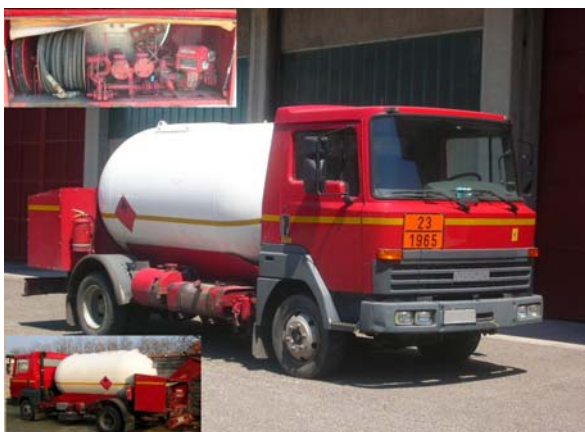
NISSAN L70 14-AC041 5.140 liters, pump, mechanic liters counters, reel hose
