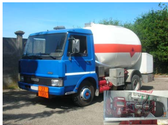
IVECO 79.14 14-AD507 7.000 liters, pump, mechanic litters counters, reel hose
