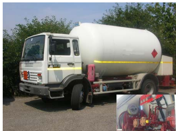
RENAULT M180 14-AJ228 13.750 liters, pump, mechanic liters counters, reel hose
