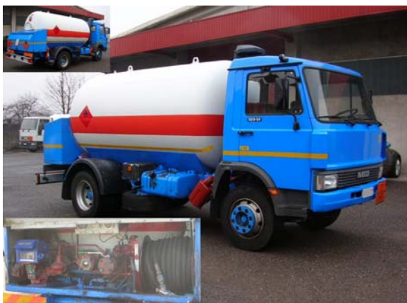
IVECO 109.14 14-NO674 7.800 liters, pump, mechanic litters counters, reel hose
