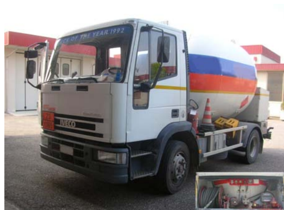
IVECO 120E23 14-FIN029 11.000 liters, pump, mechanic liters counters, reel hose
