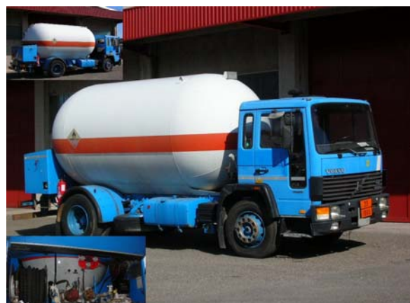
VOLVO FL616 14-AT329 15.800 liters, pump, mechanic liters counters, reel hose
