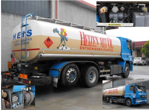
IVECO 240.42 3 axles, ABS, Retarder 15-BD139 It. 22.140 liters, aluminium tank 1 compartment, 4" bottom loading, ADR
