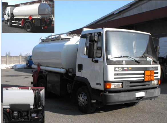
DAF 45.160 2 axles 13-AM081 It. 7.690 liters, steel tank 1 compartment, pump, tube and litter counters., ADR
