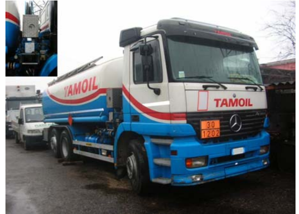
MERCEDES Actros 18.31 3 axles 13-CK689 It. 19.800 liters, aluminium tank 2 compartments, pump, tube and litter counters., ADR
