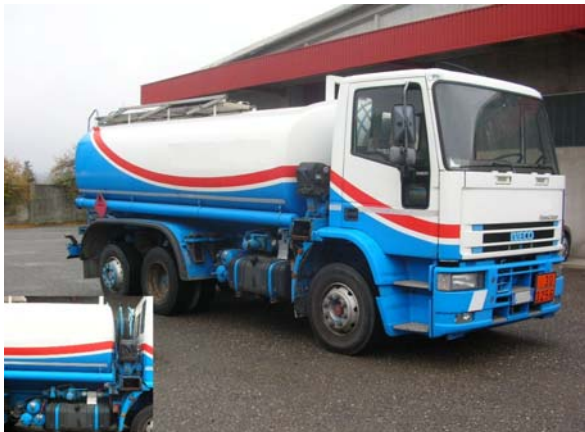
IVECO 150E27 3 axles 13-CK614 It. 13.660 liters, steel tank 1 compartment, pump, tube and litter counters, ADR.
